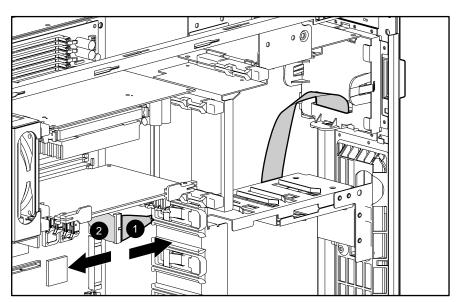
Figure 2-9. Disconnecting the IMD cable from the IMD extension cable
